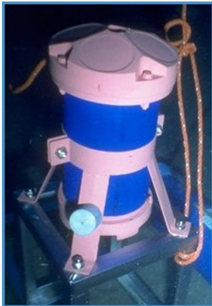
Figure 29. Antifouling Paint Applied to a WorkHorse Sentinel
