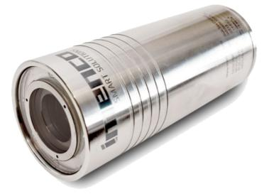
The Imenco Whitetip Shark II Colour Zoom SD Camera incorporates a 4Mpx - 1/3" CMOS sensor and features a 10x optical zoom lens. With built-in LED lights and ultra-compact and lightweight Titanium body rated to 4.000msw, it is an ideal camera for inspection of restricted spaces and for use in tooling applications.
